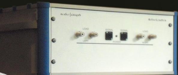
Use the AudioGraph Active LoadBox together with your existing audio measurement system - connects with USB to your computer.
