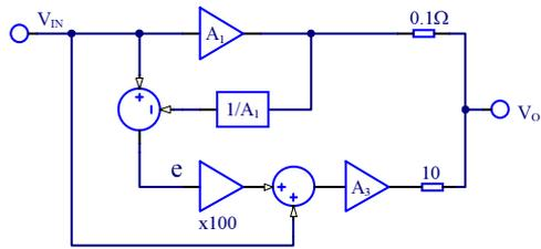
Figure 7.48 The principle of the global error feedforward amplifier that was prototyped.  $A_1$  and  $A_3$  are both simple power amplifiers. The error amplifier with a gain of 100 V/V was built using AD797 operational amplifiers.
