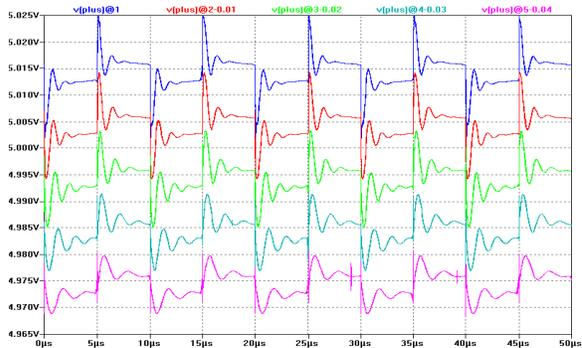
Figure 2.3(L): same as fig 2.1 but using a 2.2 $\mu$ F tantalum output cap on the +ve regulator
