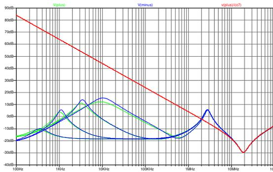
Figure 2.7(L): as figure 2.5 but with the noise bypass capacitors removed. Note the resonant peak in the audio band
