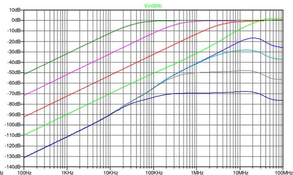
Figure 4.6(R): TI OPA350 model PSG with closed loop gain of -1 to -1000; some thought went into this one
