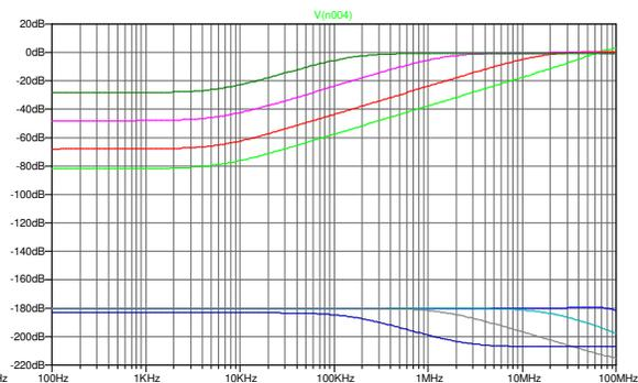
Figure 4.10(R): The Intersil (ex-Elantec) EL2227C model PSG with closed loop gain of -1 to -1000
