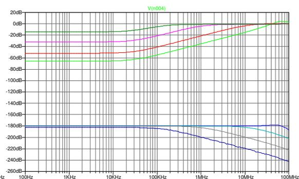
Figure 4.4(R): the closed-loop PSG for the LT1812 model.
