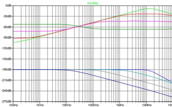
Figure 4.7(L): TI OPA627E model PSG with closed loop gains of -1 to -1000; strange pivoting at higher gains
