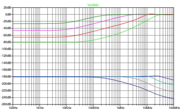
Figure 4.3(L): the closed-loop PSG for the LT1723 model, also showing the effect of finite low frequency gain
