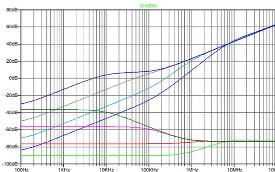
Figure 4.5(L): TI TLE2082 model PSG with closed loop gain of -1 to -1000; record-breaking GBW via supply pins
