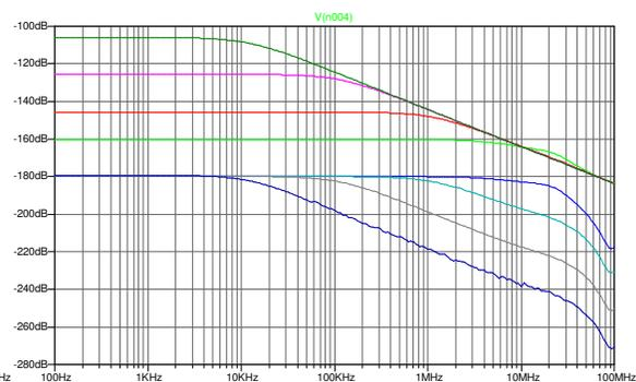
Figure 4.2(R): the open-loop PSG for the LT LT1355. Notice the dB scale
