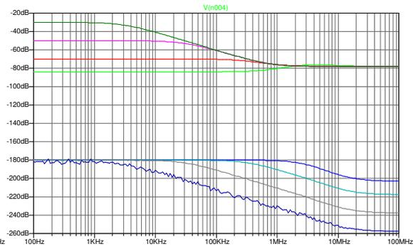
Figure 4.8(R): The TI TL072; behaviour at DC is plausible, but high frequencies are completely wrong
