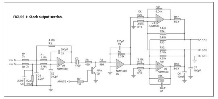
magic, this article is about improving the analog portion of the DCX, in particular the output amplifier section. This is a low cost unit, so those op amps aren't so hot, and the judicious use of electrolytic signal coupling caps (arrgh!) and—Ohm forbid!—the use of a transistor for muting means that there is much that can be done better. But, I also wanted it to be fully reversible.
