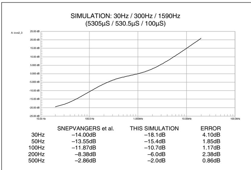
**Figure 4.** This curve was generated by a computerized circuit simulation model using turnover frequencies of 30Hz, 300Hz and 1590Hz, corresponding to time constants of 5305 $\mu$ S, 530.5 $\mu$ S and 100 $\mu$ S. The table compares the results with the data derived from the Snepvangers graph. This combination deviates significantly from Snepvangers' graph.
