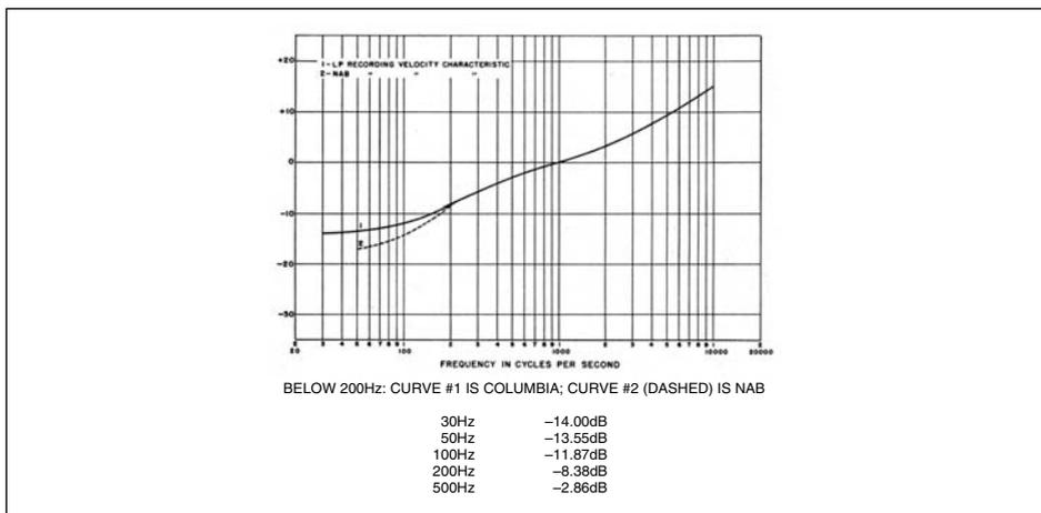
**Figure 2.** The Columbia Lp recording characteristic published by Goldmark, Snepvangers and Bachman. Below 200Hz, curve #1 is the Columbia curve. The NAB curve, from which the Columbia curve was derived, is #2. The authors failed to provide any data on the time constants or turnover frequencies used to produce the curves. The data shown for the low-frequency portion of the curve was derived by carefully measuring curve #1 using a set of precision dial calipers.
