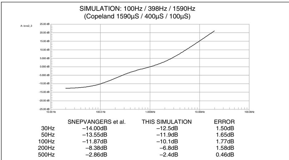
**Figure 6.** Simulation for 100Hz, 398Hz and 1590Hz (1590 $\mu$ S, 400 $\mu$ S and 100 $\mu$ S), a combination suggested by Copeland. Errors are less than 2dB.
