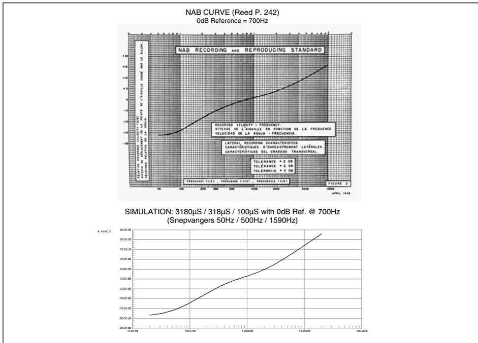
**Figure 9.** The NAB graph, published by Reed, is shown in the top illustration. NAB put the 0dB reference at 700Hz, rather than at the customary 1kHz, which has caused considerable confusion over the years. The bottom graph is a simulation of the NAB curve using 50Hz, 500Hz and 1590Hz (3180 $\mu$ S, 318 $\mu$ S and 100 $\mu$ S). The 0dB reference in the simulation has also been placed at 700Hz, to allow meaningful comparisons to the NAB graph.
