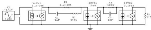
Columbia Lp Curve Simulation: 100Hz/500Hz/1590Hz (+16dB @ 10kHz)
