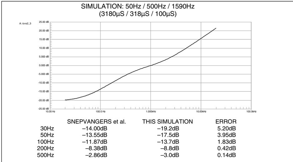
**Figure 5.** Simulation for 50Hz, 500Hz and 1590Hz (3180 $\mu$ S, 318 $\mu$ S and 100 $\mu$ S). Errors at the lowest frequencies are significant.
