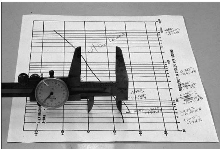
**Figure 3.** Measuring the Snepvangers graph using precision dial calipers.
