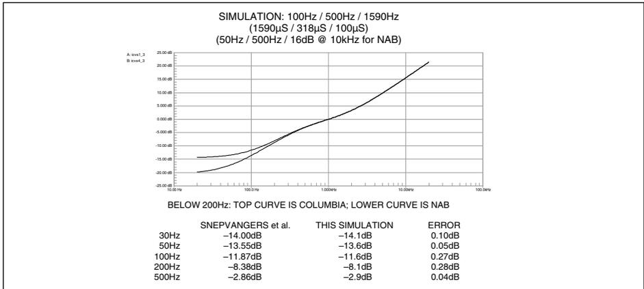
**Figure 8.** Simulation for 100Hz, 500Hz and 1590Hz (1590 $\mu$ S, 318 $\mu$ S and 100 $\mu$ S), as suggested by Eargle and others. This combination produced the lowest errors when compared to Snepvangers' graph indicating, beyond a reasonable doubt, that these are the correct turnover frequencies and time constants for the Columbia Lp equalization curve.
