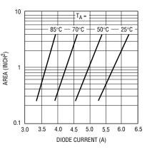
Figure 4. Maximum diode current vs PCB area
