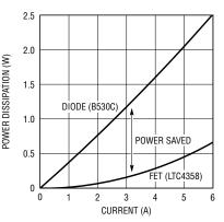
Figure 2. The LTC4358 ideal diode takes on a 5A B530C Schottky diode. The LTC4358 easily wins in voltage drop, power loss and package size.
