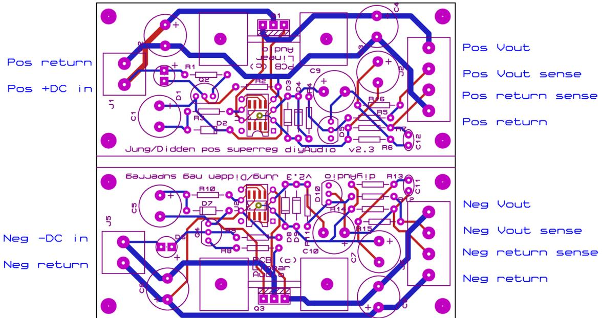
Figure 2 - PCB layout and connections
