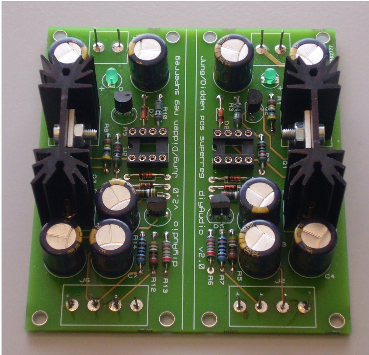
Figure 4 – prototype V 1 superreg (without recommended PCB screw terminals). V2.3 has same form factor and pretty much the same layout.
