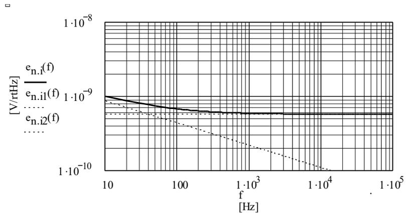
Figure 20 Trace of the calculated input referred noise voltage density of 2SC2647E, incl. its tangents (dotted)
