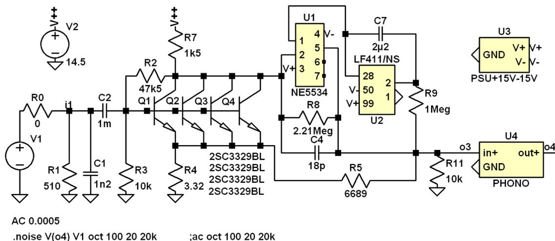
Figure 22 Simulation schematic to get the input referred figures shown in Tables 3 & 4
