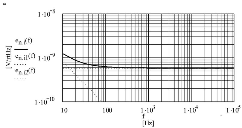
Figure 21 Trace of the calculated input referred noise voltage density of 2SA1085E, incl. its tangents (dotted)
